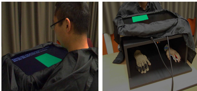
Fig. 1. Experimental setup. Participants wore an orientation tracker and a data glove on their right hand, and SCR remote transmitter on their left hand, the cloth served to cover the area between screen and participants.
